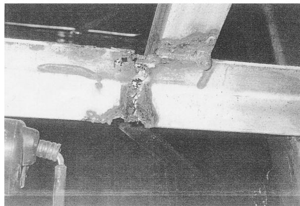
(a) Inner side of corroded hot water tank
